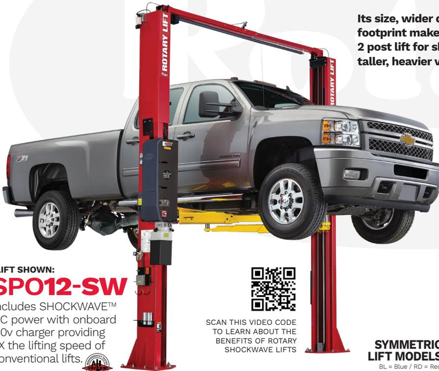
Its size, wider drive-thru and larger footprint make the SPO12 the optimal 2 post lift for shops that work on taller, heavier vehicles.
